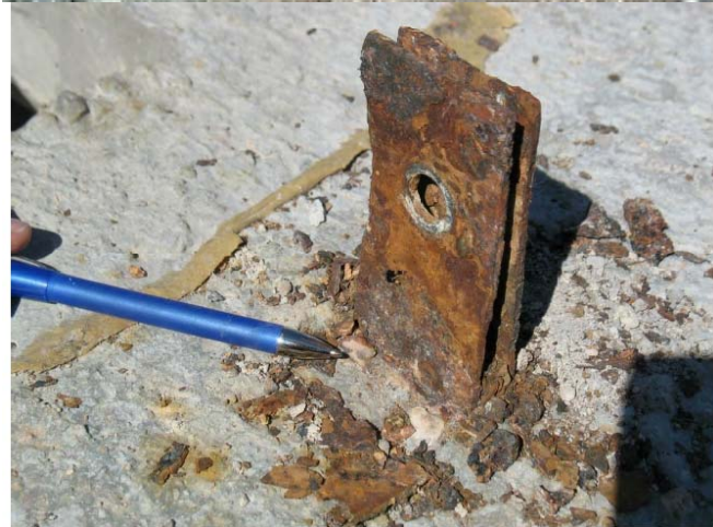
Figure 50. Cheyenne MSE Wall Corrosion Investigation - Corroded Steel Facing Connecti
